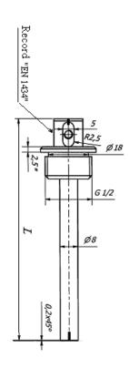
Pocket and probes' drawing can change without any notification.
