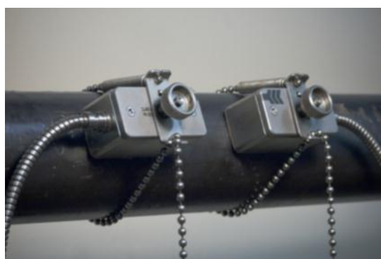
Illustration 5: Sensor mounting with fixtures and chains
