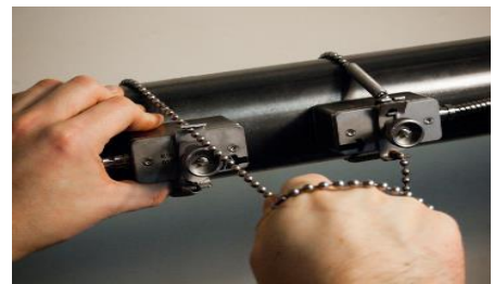
Illustration 4: Sensor mounting with clips and chains
