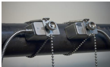
Illustration 4: Sensor mounting with clips and chains
