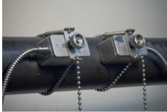
Illustration 6: Sensor mounting with fixtures and chains
