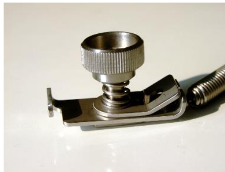
Illustration 7: Sensor mounting with fixtures and chains (retaining clip)
